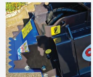
Hydraulic hoses and motor well protected inside the frame
